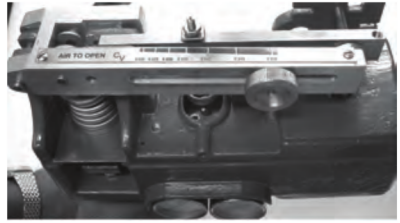
Figure 4: Adjusting Cv for each plug /seat ring combination
