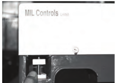
Figure 9. Adding a Packing Ring
