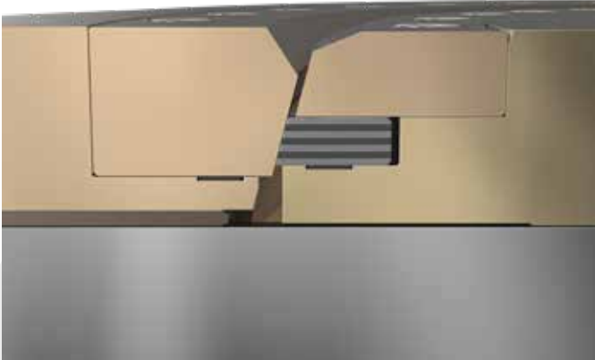
Image 3. Conical, metal to metal seating design.
