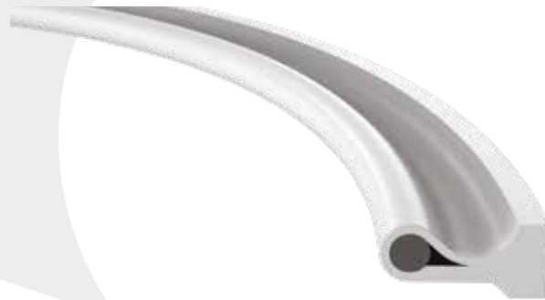
Image 3. Soft seat design, RPTFE jacket and elastomer energiser
