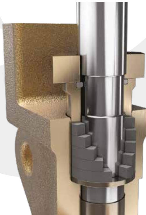
Image 2. Graphite packing arrangement
