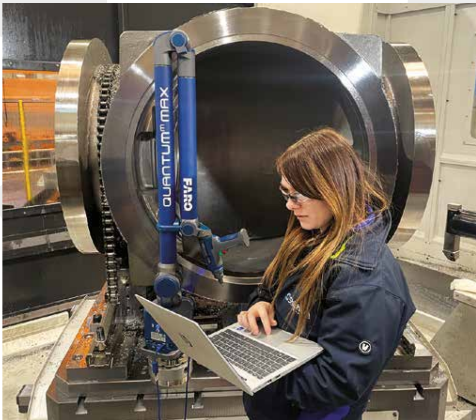
Distance inspection checks during the machining of a 24" Swing check valve body
