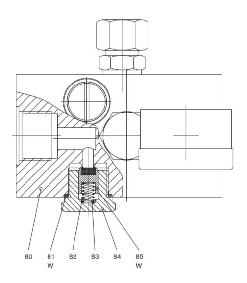
parts marked W are to be kept in stock for maintenance.
