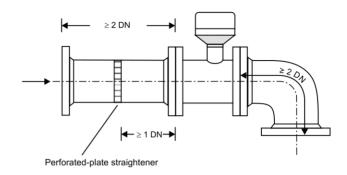
In each case, a 2 DN inlet pipe and a 2 DN outlet pipe are required, while also a bend may be used as outlet pipe. If flow perturbation (e.g. due to a gas pressure controller) occurs upstream of the inlet pipe, it is additionally necessary to use a perforated-plate straightener. There are perforated-plate straighteners available complying with ISO 5167-1 or of the type RMG LP-35, the latter resulting in a pressure loss which is 2.5 times lower than that of the standardized flow straightener.
