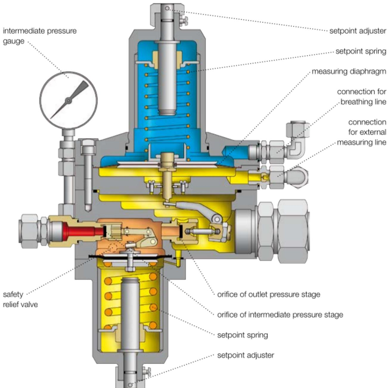
The gas pressure regulator RMG 201 is designed to keep the outlet pressure constant within given limits, independent of inlet pressure and/or flow deviations.
