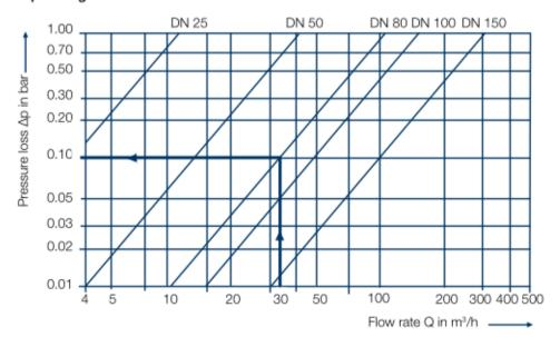
**Example:** nominal width DN 80, flow rate Q = 35 m<sup>3</sup>/h -> pressure loss  $\Delta p = 0.1$  bar
