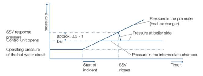
The safety shut-off device (SSV) will open again when the pressure in the heat exchanger (above the valve plate) has fallen to a value below the response pressure of the control unit (SSV response pressure minus 0.3 to 1 bar). The remote indication system is available in two different designs depending on the temperature in the hot water circuit. It cannot be retrofitted.
