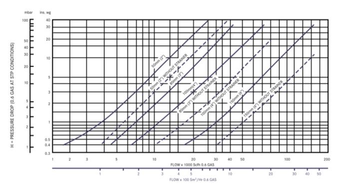
Valve Maximum Capacity Gas Velocity based on nominal pipe sizes, must not exceed 75m/s (245 ft/s). At S.T.P. Conditions the pressure drop may be obtained directly from the graph. For other pressure conditions the following formulae apply:
