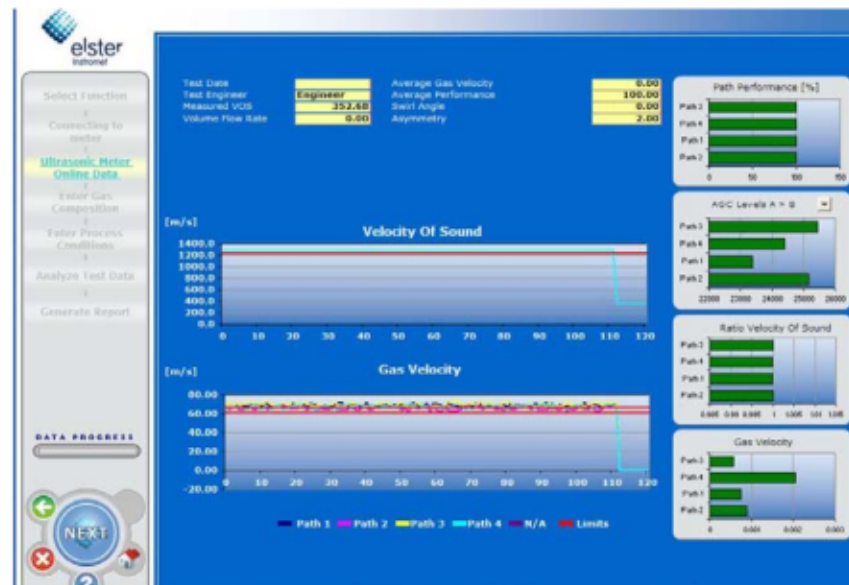
Figure 2-4: Ultrasonic Meter Online Data
