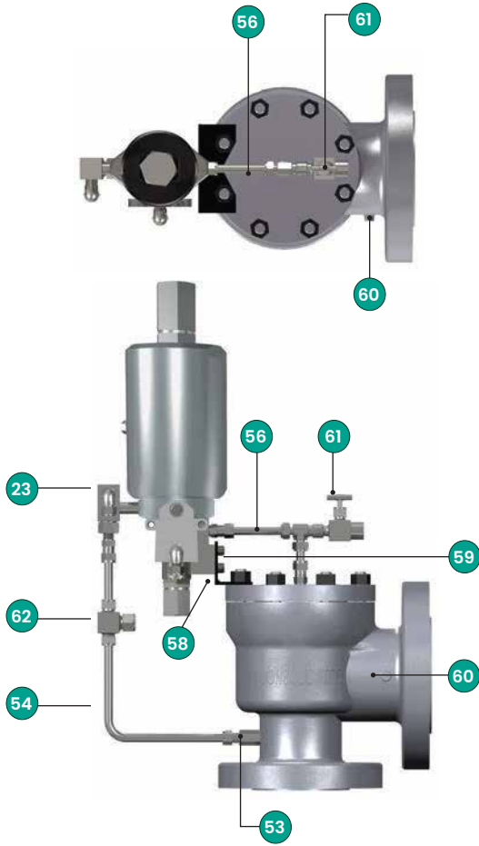
Pilot Valve with Manual Blowdown and Pilot Supply Filter (Standard for Steam Applications) (Optional for Liquid and Gas Applications)
