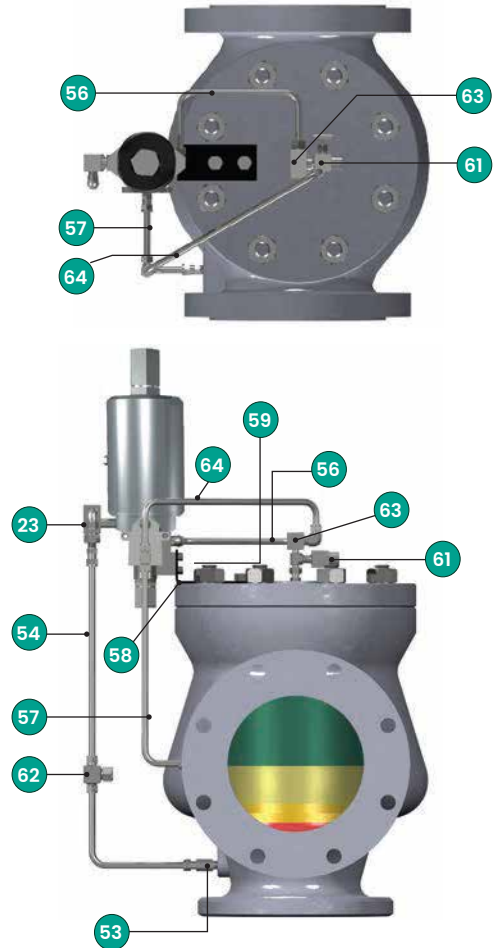
Pilot Valve with Manual Blowdown, Pilot Supply Filter and Backflow Preventer (Optional For Steam Applications)
