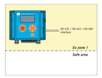
The EC 911 version is exclusively supplied by a lithium battery and has been approved for Ex zone 1 as an intrinsically safe device.
