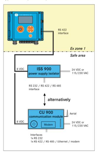
The EC 912 version has been approved for Ex zone 1 as an intrinsically safe device. The boards of the EC 911 and EC 912 are identical to each other; they differ in that the battery of the externally supplied EC 912 serves only as an emergency battery.
