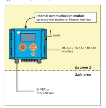
The EC 922 version is intended for use in Ex zone 2; it is not permissible to operate this device in Ex zone 1. It is externally supplied and includes a power pack (24 VDC or 115/230 VAC). A lithium cell serves as an emergency battery to supply the volume corrector. However, it does not supply the internal communication module.
