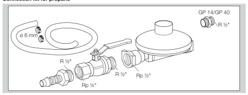
Pressure reducer, manual valve, hose (length = 2 m), 2 hose clamps, R  $\frac{1}{2}$ " double nipple for GP 14/GP 40, to connect the gas combination control CG to the gas supply, Order No.: N52600025
