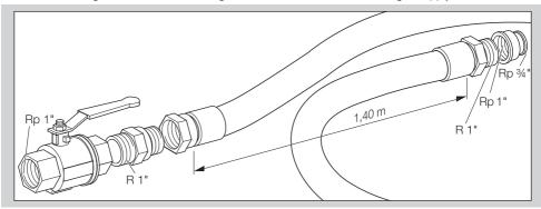
Connection kit: R 1" threaded connection, total length = 1.50 m + reducing socket Rp 1 – Rp %", Order No.: N52600071
