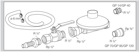
Pressure reducer, manual valve, hose (length = 2 m), 2 hose clamps, R  $\frac{1}{2}$ " double nipple for GP 14/GP 40, R  $\frac{1}{2}$ -Rp  $\frac{3}{4}$ " reducing fitting for GP 70-GP 120, to connect the gas combination control CG to the gas supply, Order No.: N52600025
