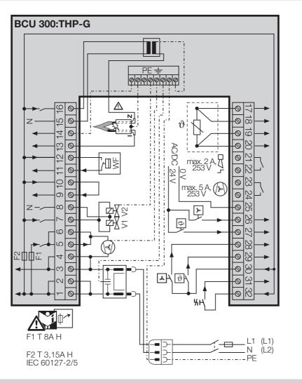
In order to ensure post-cooling, the heater constantly requires 230 V AC.
