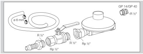
Pressure reducer, manual valve, hose (length = 2 m), 2 hose clamps, R ½" double nipple for GP 14/GP 40, to connect the gas combination control CG to the gas supply, Order No.: N52600025
