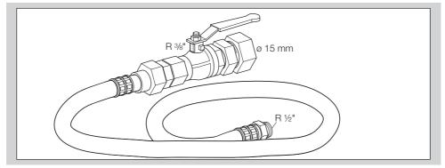
Manual valve and hose (DVGW certified, length = 2 m) to connect the gas combination control CG to the gas supply, Order No.: N52990209
