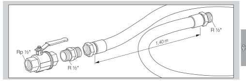
Connection kit: R  $\frac{1}{2}$ " threaded connection, total length = 1.50 m, Order No.: N52600073 Connection kit for propane
