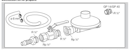
Pressure reducer, manual valve, hose (length = 2 m), 2 hose clamps, R ½" double nipple for GP 14/GP 40, to connect the gas combination control CG to the gas supply, Order No.: N52600025
