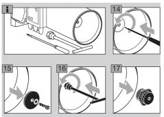
The spark electrode and flame rod can be removed without having to dismantle the burner chamber.
