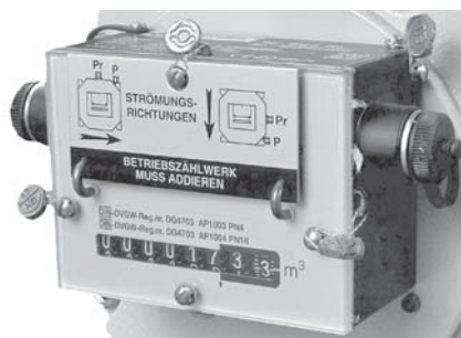
Flow direction: left - right respectively. top - bottom
